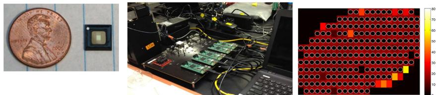
**Automated Nanopore Array Setup:** In 3 automated steps, the 264 sensor IC electrodes are first coated with lipid and salt solution to create bilayers, pore solution is added to insert single pores, and when the pores are ready, the remaining reagents are added to initiate sequencing. Shown are photographs of the chip, the device and a heat map of 200 single pores over an array of sensors. Black circles represent single pores over single sensors.
