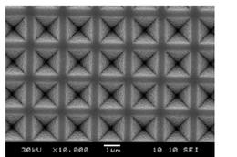
Scanning electron micrograph of Au-coated, lithographically patterned substrate - Klarite.
